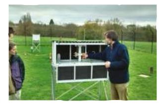
Ozone pollution is monitored by taking a sample of air into an analyser, which shines specially produced light through the sample inside a tube. A measurement of how much light is absorbed is proportional to the concentration of ozone in the air.
